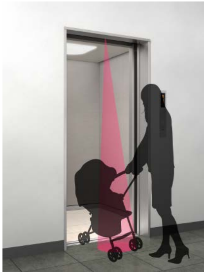
Hall Motion Sensor: HMS (Optional)
